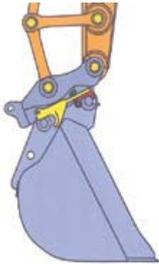
(d) Hydraulic ram is sent forward to retain rear pivot pin - note that auto-lock remains on front pivot pin
